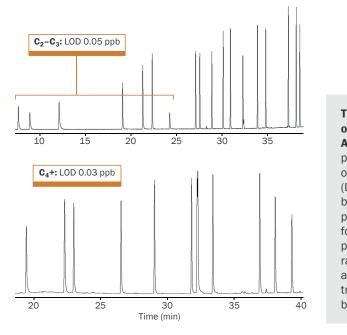
The efficient operation of the Air Server-xr provides limits of detection (LODs) well below the 0.5 ppb required, for ozone precursors ranging from acetylene to trimethylbenzene.
