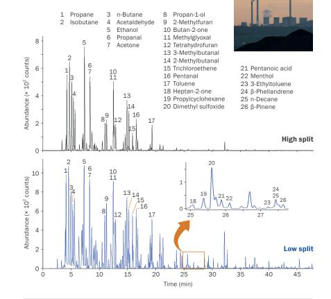
Markes' sample splitting and re-collection technology allows samples such as this odorous industrial air to be re-analysed. As well as aiding method validation and offering greater peace-of-mind, it also allows a single sample to be analysed at different split ratios, allowing both highand low-concentration components to be accurately quantitated.
