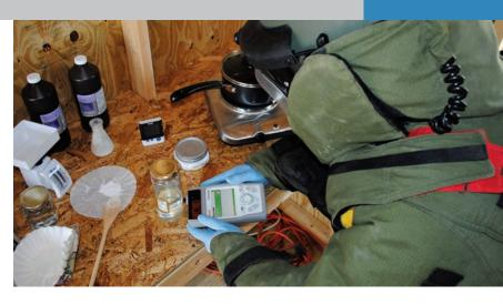
The Thermo Scientific FirstDefender RM instrument is a rugged Raman spectrometer for rapid, accurate identification of unknown chemicals directly in the field. At 1.8 pounds (800g), the FirstDefender RM analyzer includes a large, vivid display for ease of use in bulky protective gear and can be easily transported into a hazard zone.
